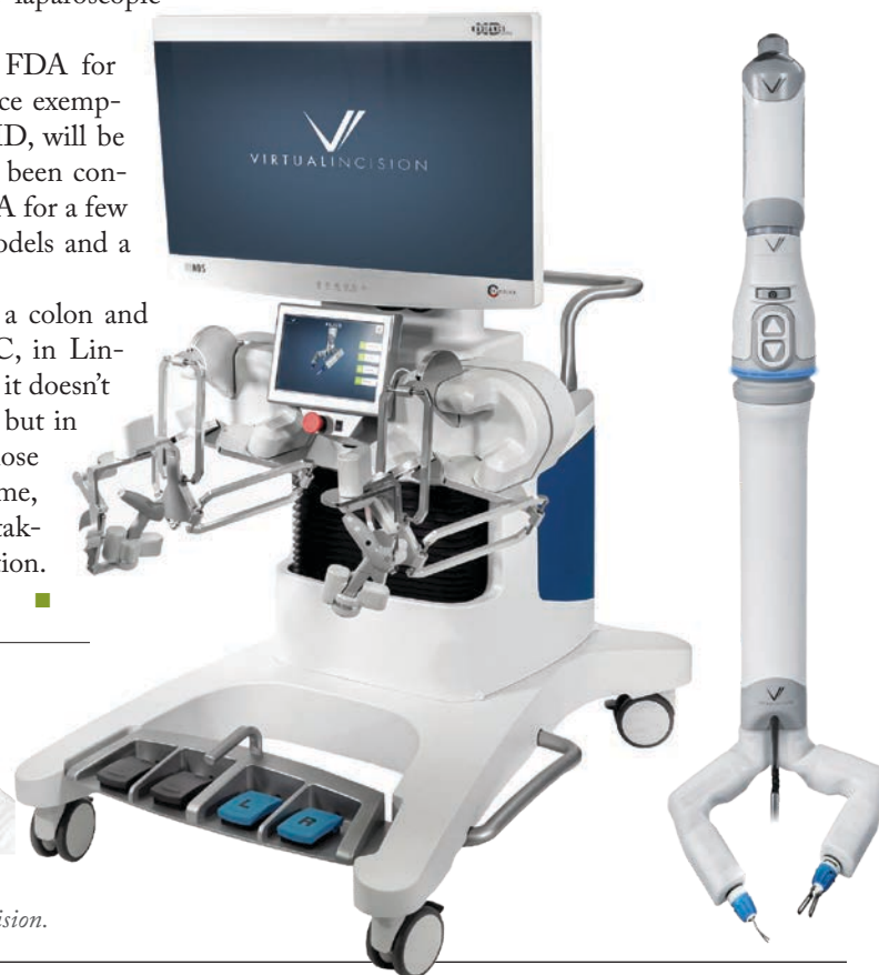
The miniaturized in vivo robot assistant (MIRA) consists of an articulating scope with two miniaturized arms (lower right) and a surgeon console (above and below).
