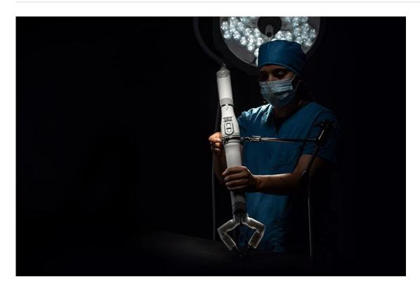
Virtual Incision, a company based in Lincoln, Nebraska, has developed the miniaturized *in vivo* robotic assistant (MIRA) platform to perform minimally invasive abdominal surgeries, such as colon resections. Conceived as a small and accessible surgical robotic support device, the miniaturized system is considerably less expensive than current robotic surgical platforms.
